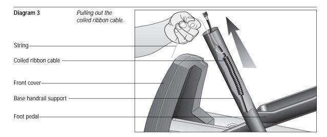
CAUTION: Do not let go of the string until you are holding onto the coiled cable. The string could drop inside the base support making it difficult to retrieve the coiled ribbon cable.
